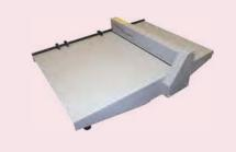
Available in both 14" and 20.5" widths, this foot pedal operated machine increases the speed of production over a manually operated machine. As an added feature, with the turn of a dial the crease width is adjustable from a 1.2 mm profile crease (for text weight stocks under 150 GSM) to the wider 1.6 mm profile crease for substrates as thick as 350 GSM
