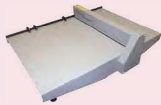
Available in both 14" and 20.5" widths, this foot pedal operated machine increases the speed of production over a manually operated machine. As an added feature, with the turn of a dial the crease width is adjustable from a 1.2 mm profile crease (for text weight stocks under 150 GSM) to the wider 1.6 mm profile crease for substrates as thick as 350 GSM.
